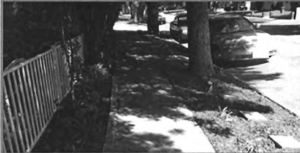
AFTER: Photo of the same area with permeable decomposed granite path, drought tolerant plants, and mulch to retain water.
