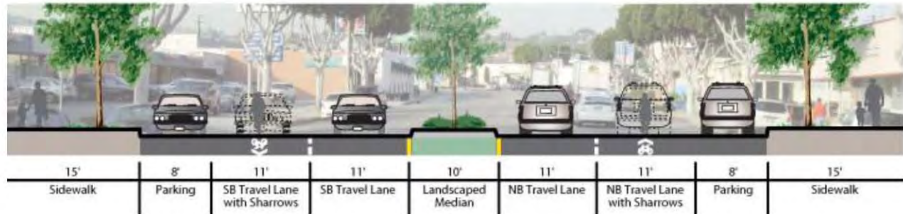
Figure 5-3: Typical Garfield Avenue Cross Section
