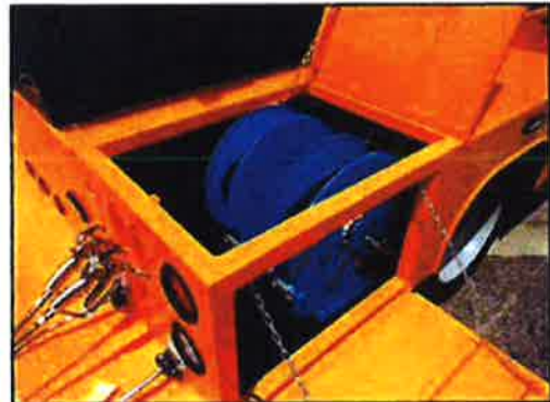
Hose reels mounted below deck with top and side doors for easy maintenance.
