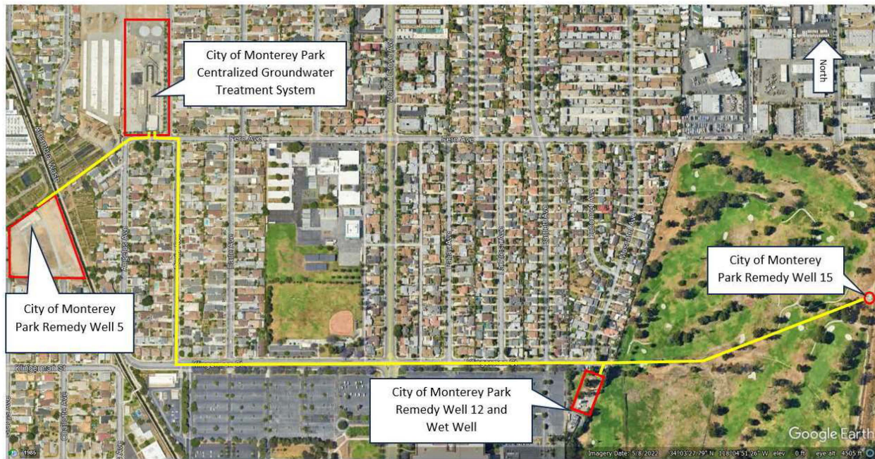
Figure 3: CMP Centralized Groundwater Treatment System
